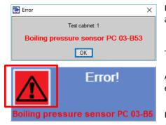
If a cabinet has an **error**, an error message indicating the cabinet number and the error is displayed.
