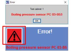
If a cabinet has an **error**, an error message indicating the cabinet number and the error is displayed.
