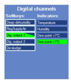
The digital channels display relates to the test cabinet currently displayed. Depending on the cabinet configuration (how many digital channels this cabinet has), the softkeys and indicators are displayed dynamically. In this area, only those digital channels are displayed which are actually present in the control system and released for display. There are two types of digital channels:
