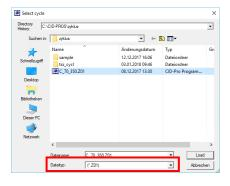
Here, already created programs can be opened and loaded into the editor module. To do so, the desired file must be selected from the list and Load must be confirmed.
