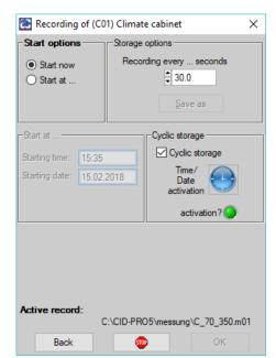
Also in the status overview, the activated cyclic storage is displayed in the upper bar, which in its turn is indicated by a **green LED**. The days, hours, minutes and seconds are displayed until the next storage.
