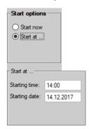
In addition to starting immediate recording, a delayed start can also be activated. The **Starting time / Starting date** are entered via the keyboard. Any permitted date within one year can be entered. The time must keep the hh:mm (hour:minute) format. If the predefined formats are not met, the entry is ignored.
