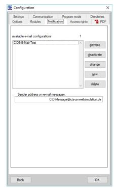
The **Notification** menu item allows e-mail messages which are automatically sent by the **CID-PRO 5** software to be set up and activated.
